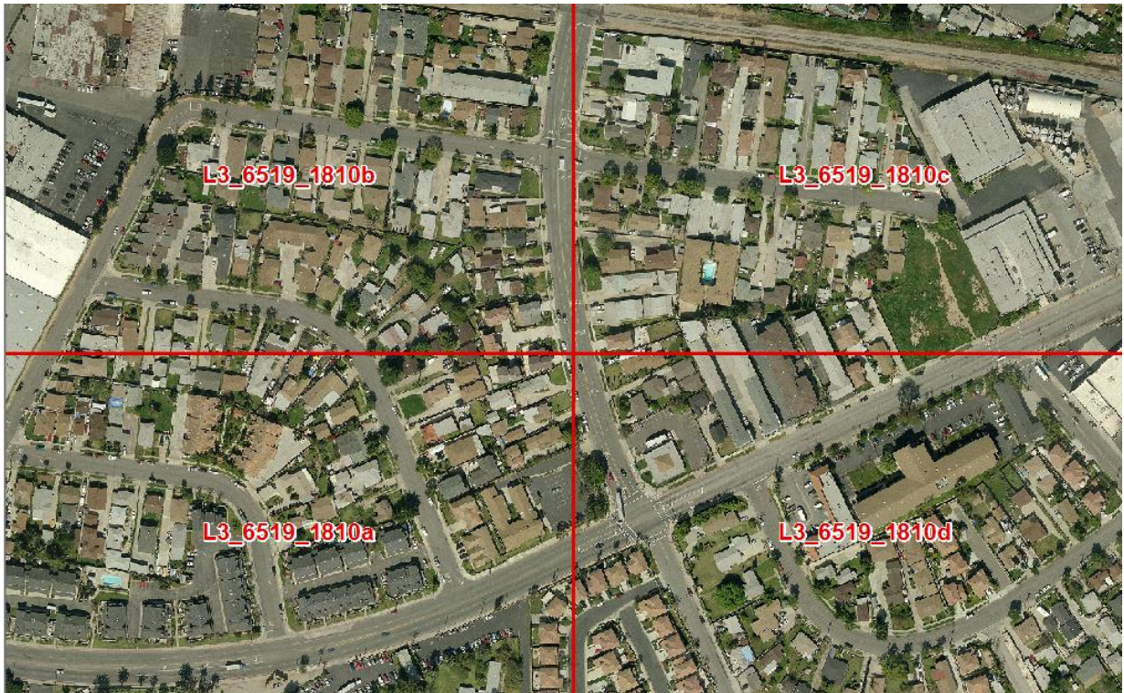
Sample 4-inch tiles with the LAR-IAC3 tile grid and naming convention.
